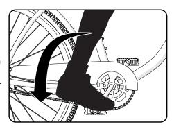
If your bicycle has a caliper brake(s) in addition to the coaster brake, always use the coaster brake as the main brake to stop the bicycle.
