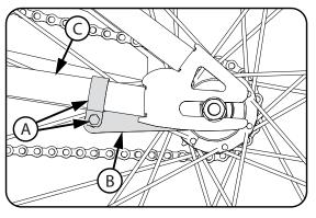
• Every time the bicycle is ridden, make sure the clamp (A) on the brake arm (B) is securely attached to the chain stay (C) of the bicycle frame. The coaster brake will not work correctly if the brake arm is not attached to the chain stay.
